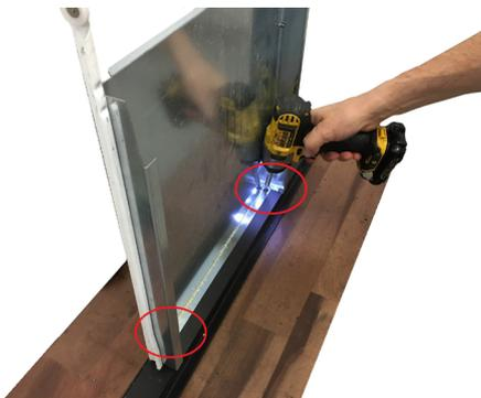
Fig. 36 - Removing the front panel
