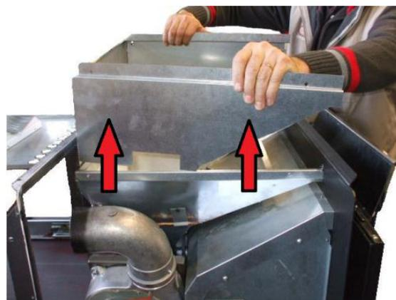
Fig. 60 - Casing removal
