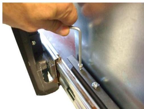
**Fig. 15 - Insert fixing rear screw**
