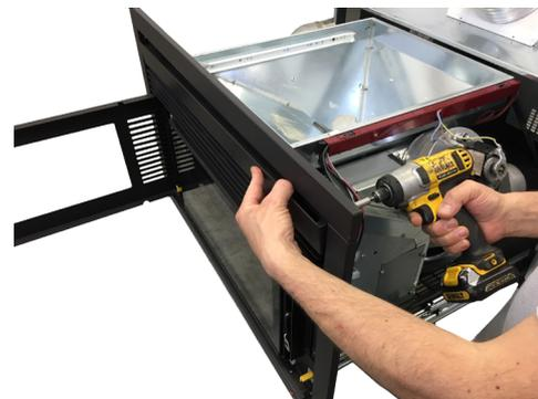
Fig. 37 - Securing the front panel
