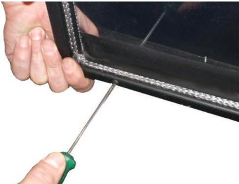
Fig. 55 - Screw removal
