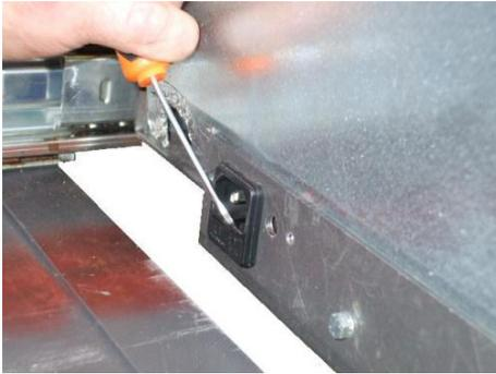
*Fig. 63 - Fuse removal into the electric socket*
