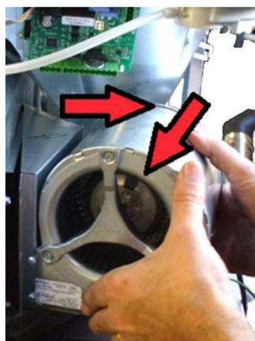
Fig. 62 - Fan removal
