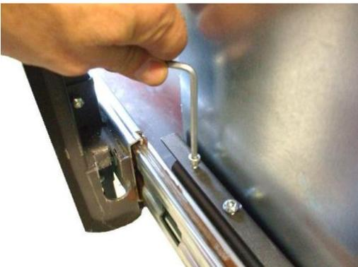
Fig. 20 - Insert fixing rear screw
