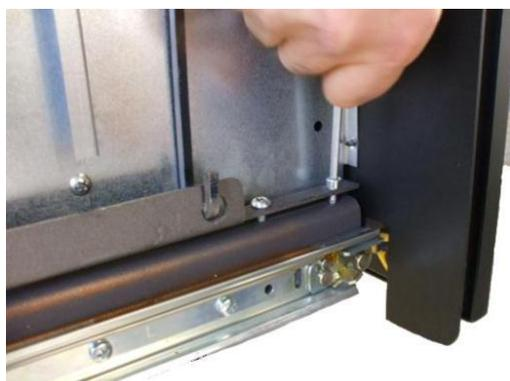
**Fig. 14 - Insert fixing front screw**
