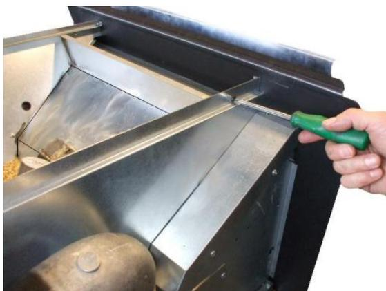
Fig. 59 - Unnscrew casing screws
