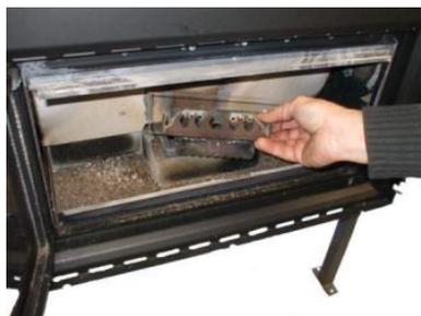
**Fig. 39 - Burning pot removal**
